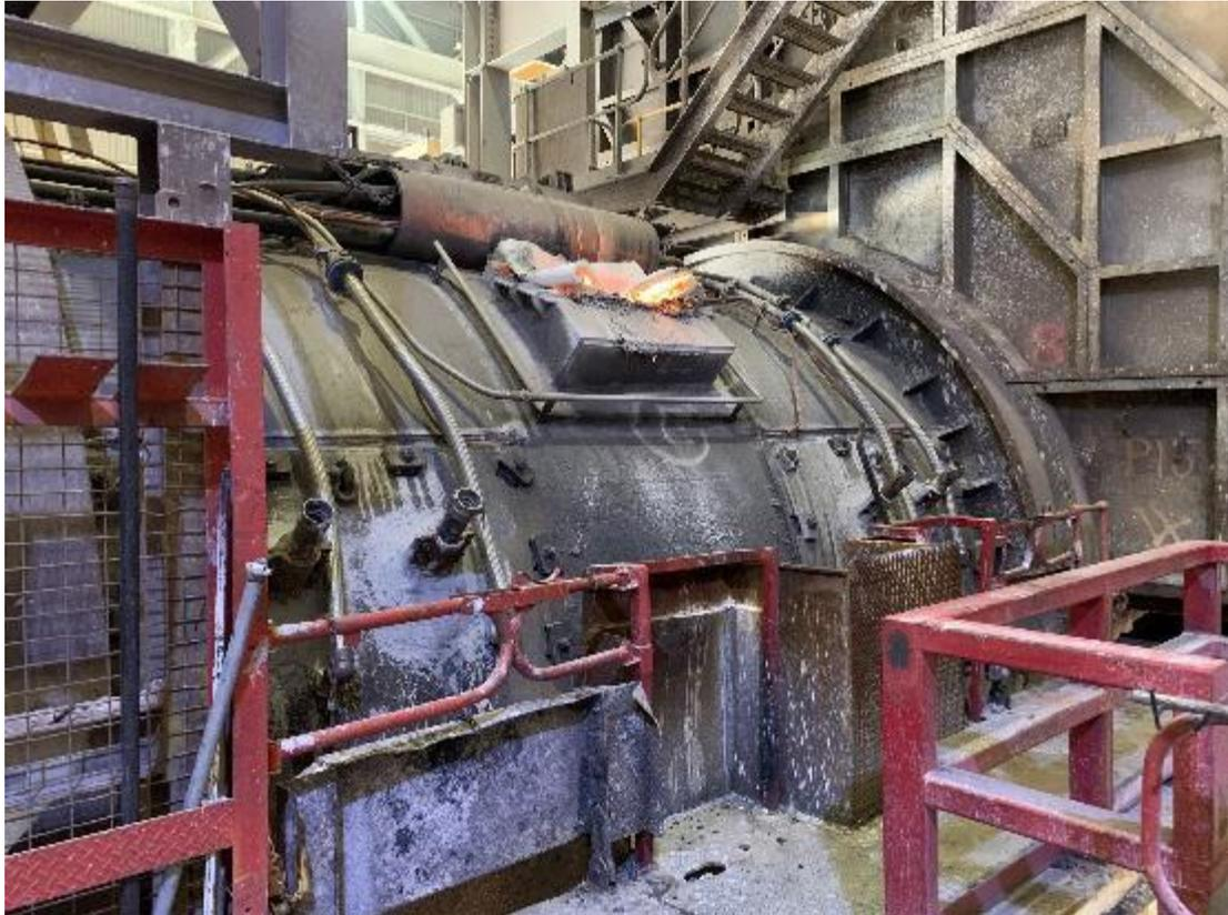
Anode furnace for pyrometallurgical refining
